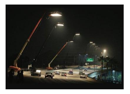
2. Example of height and beam angle of lighting fixture mounted upon boom lifts for night exterior shooting. (Example only for illustrative purposes, not part of the lighting design proposed for this application)
